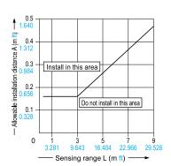
Note: The effective aperture angle for this device is ±2.5° or less (when L > 3 m 9.843 ft) as required by IEC 61496-2, ANSI/UL 61496-2. However, install this device away from reflective surfaces considering an effective aperture angle of ±3° to take care of beam misalignment, etc. during installation.
