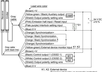
K1, K2: External device (Forced guided relay or magnetic contactor)
