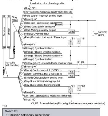
For automatic reset 0 to +1.5 V (source current 5 mA or less): Emission, Open: Emission halt
