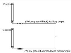
The diagram at left shows the configuration when using NPN output, interlock function "disabled (automatic reset)" and external device monitoring function "enabled".
