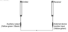
It is also possible to set the external device monitoring function into invalid by using the handy-controller SFB-HC (optional). Refer to instruction manual enclosed with this product for details.
