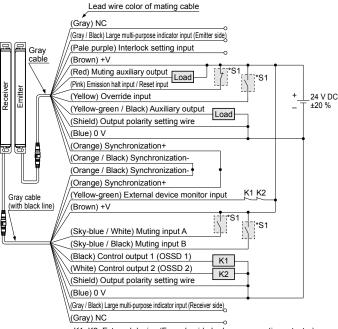
K1, K2: External device (Forced guided relay or magnetic contactor)
