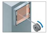
The floating blanking function allows to disable up to three unspecified beam channels. Control output (OSSD) will not turn off as long as the number of interrupted beam channels is less than the set number of beam channels. This function is convenient when an obstruction moves inside the detection area during setup changes or when loading materials within the detection area of light curtain. \*The min. sensing object will change when the floating blanking function is used.
