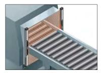
The **SFB-HC** handy-controller provides a fixed blanking function that prevents control output (OSSD) from turning off even if certain beam channels are interrupted. This function is convenient for applications where an obstacle always interrupts certain beam channels. Additionally, it is safe since control output (OSSD) is forcibly turned off in the event the obstruction moves outside the detection area.
